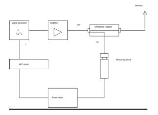
Particularly for propagation measurements, field strength and frequency of specific transmitters are to be measured frequently or continually over a longer period of time. ALC is of great advantage in this case and improves the accuracy of field-strength measurements and reproducibility. In the above example the level can be kept constant within certain limits.
